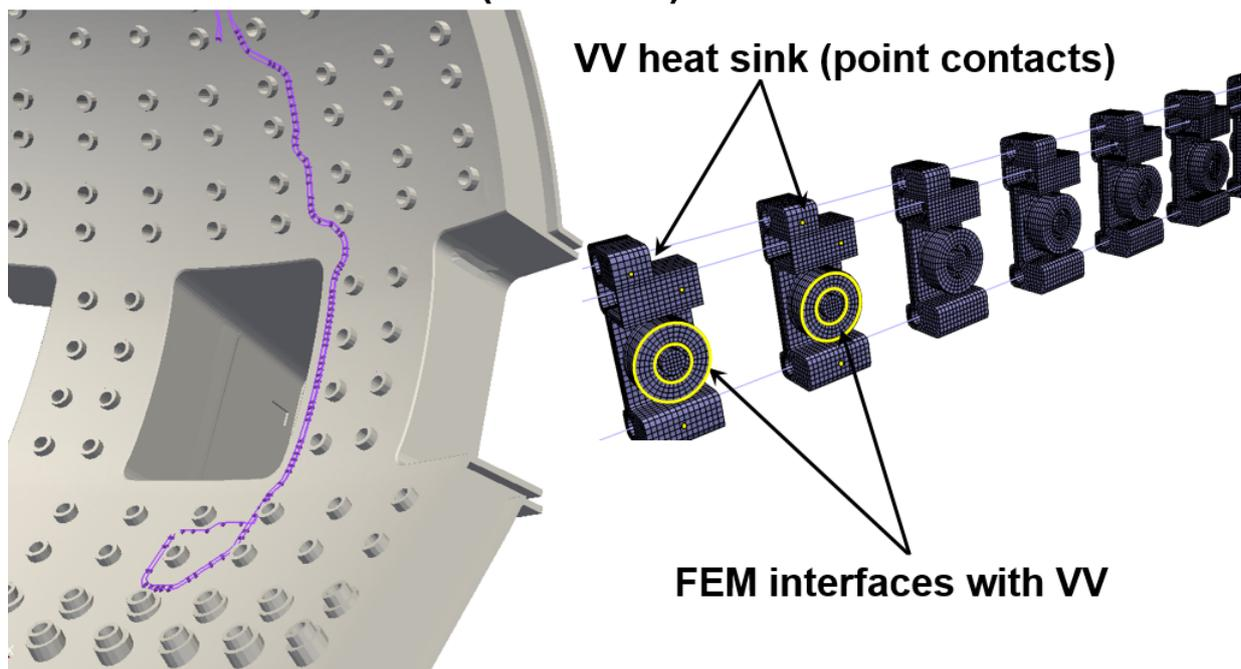
Figure 1: Thermal generic model of a typical in-vessel system.
