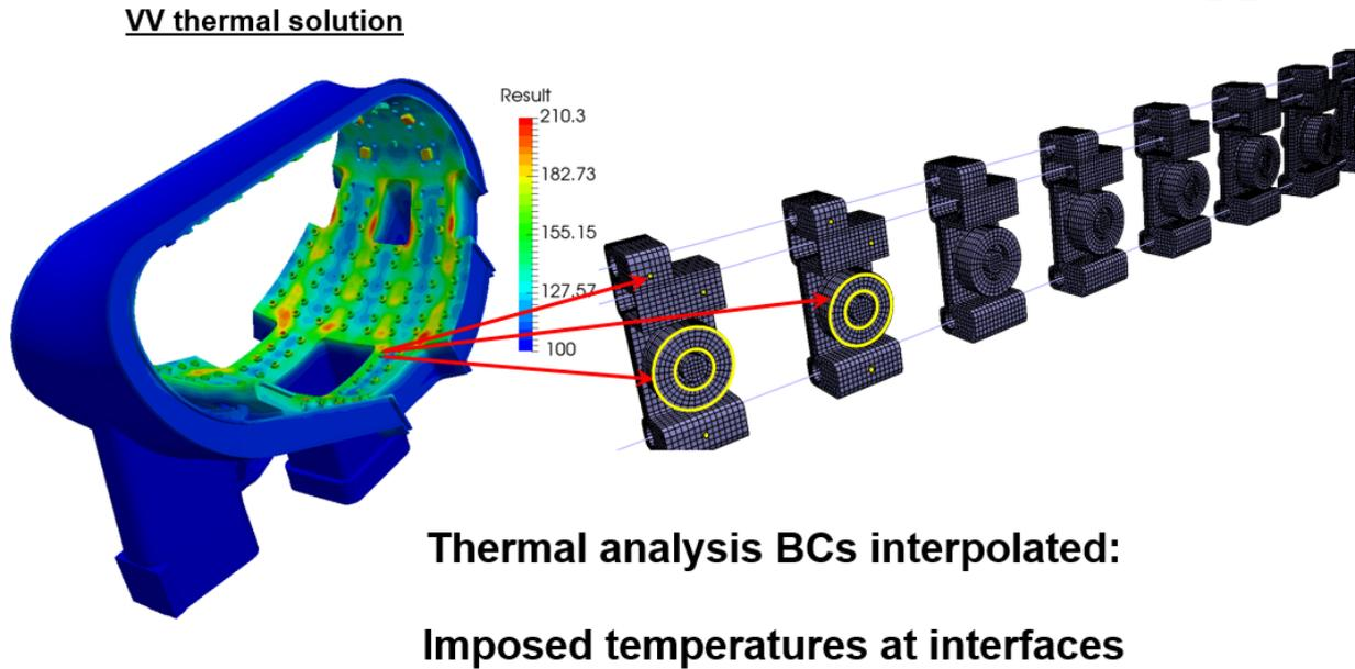
Figure 2: Thermal interface loads for a generic model of a typical in-vessel system.
