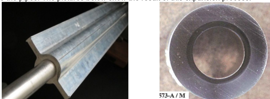
Figure 7 – General view of the 4 K cryopanel, before charcoal coating and polishing, and its cross section
