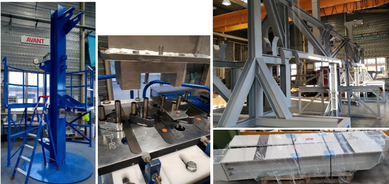
Figure 15 – Some of the tooling used during the assembly, testing and transportation of the Mitica Cryopump. On the left side: the pumping sections assembly tool; on the middle: the cryopanel-TRS centring tools; on the right side: the subframes and cryopump assembly tools.
