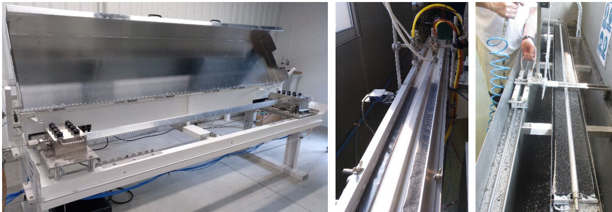
Figure 16 – Some of the tooling used during the expansion and charcoal coating of the panels. On the left side: the pipe expansion station; on the middle: the glue spray station; on the right side: the charcoal coating station.
