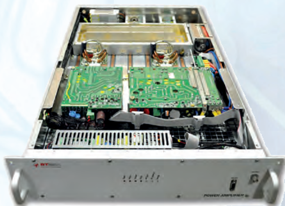
hot-plug liquid-cooled PA module 2kW
