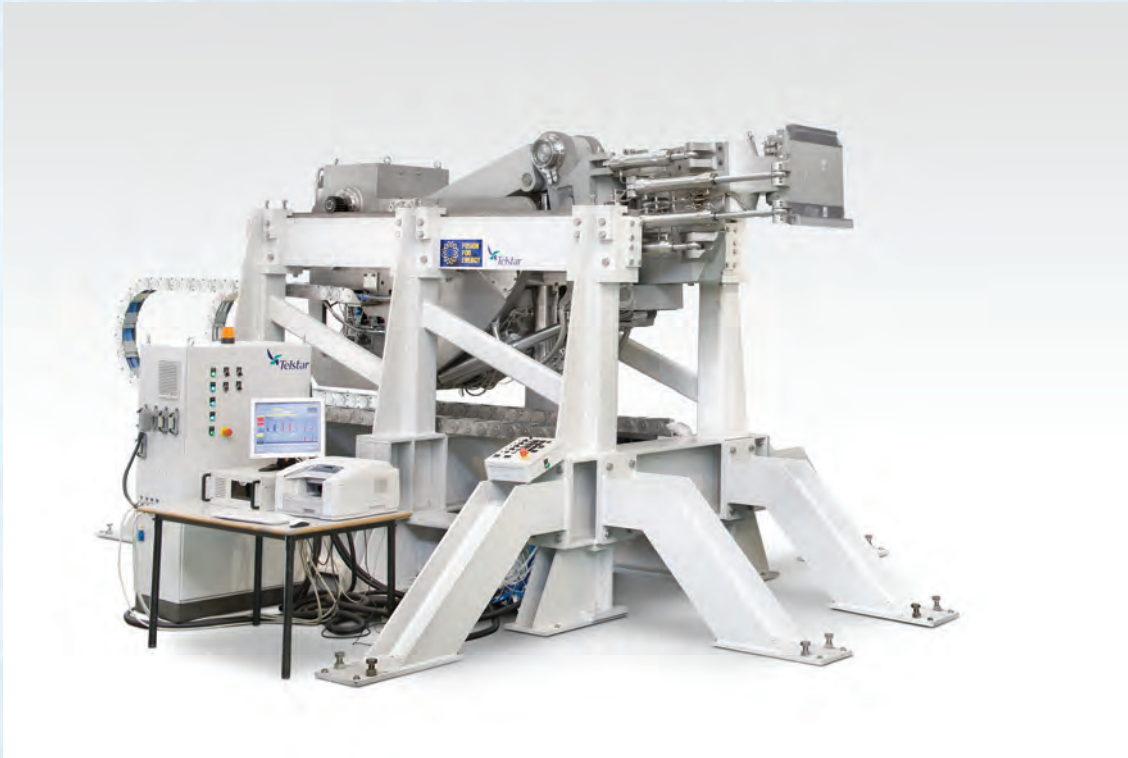
Divertor RH Cassette Multifunctional Mover (CMM) and Second Cassette End Effector (SCEE) prototypes on a test stand
