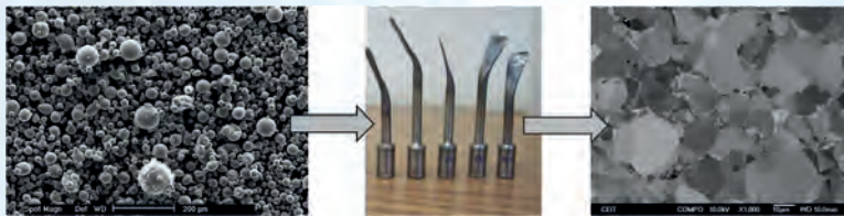
Oxide Dispersion Strengthened Ferritic Steels (ODS FS) obtained by PM route, avoiding Mechanical Alloying
