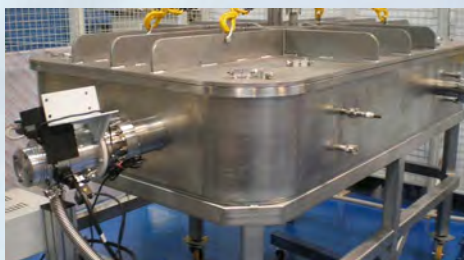
Cryostat for testing superconducting coils at 10K
