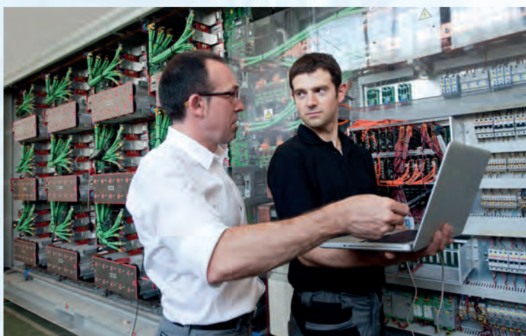
HV Solid State Klystron Modulator: 85kV, 160A, 14 MW peak, 1.5ms pulse, 60Hz repetition rate. ESS Bilbao (Spain) and SNS Oak Ridge National Laboratory (USA). © JEMA
